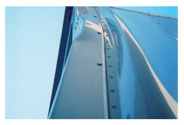
Van trailer damaged from backing.
